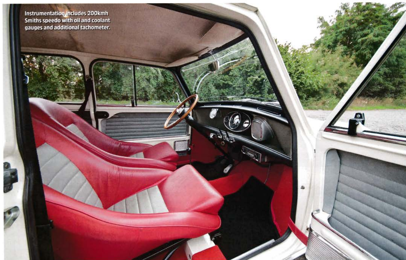
15-inch wood-rimmed Formula three-spoke steering wheel.
