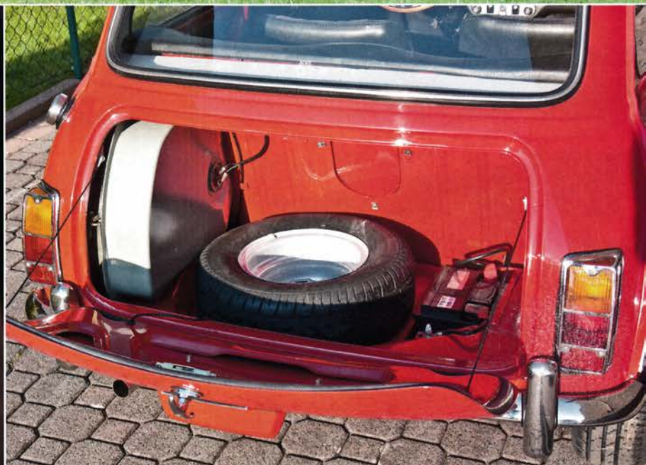
Authi logos can be found on everything, even the keyring. Right: Boot houses a 5.5 gallon fuel tank, Rostyle spare and the battery with FEMSA terminal clamps.
